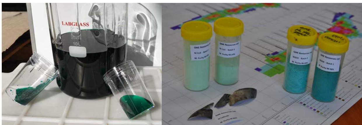
Pure Ni Sulphate (Electrolyte) Solution generated from the DSX continuous pilot plant.
