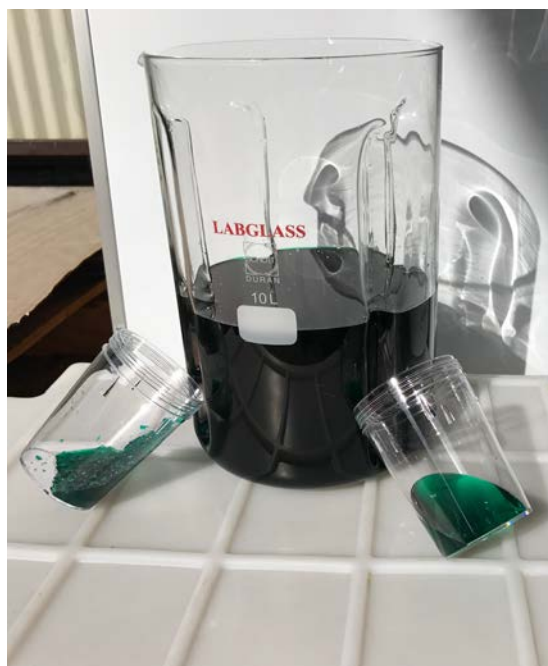
Photo 3: Pure Ni Sulphate (Electrolyte) Solution generated from the DSX continuous pilot plant. Left hand beaker shows naturally occurring Ni Sulphate crystals that crystallise out of the saturated Ni sulphate solution.
