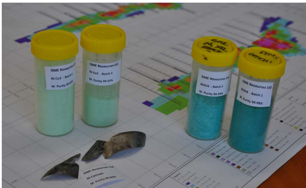
Photo 1 : High purity (+99.95%) Nickel products produced from the NiWest continuous pilot plant.
