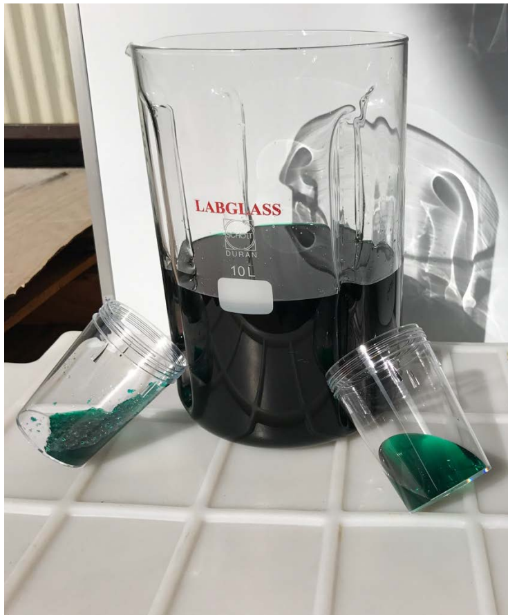
Figure 2: Pure nickel sulphate (electrolyte) solution (~5L) generated from 24 hours operation. Left beaker shows naturally occurring nickel sulphate crystals that crystallise out of the saturated solution.
