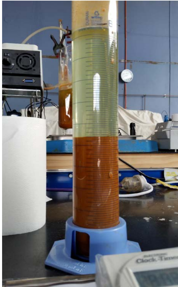
Figure 2: Results of solution neutralisation and Fe/Al removal batch test, showing excellent solid/liquid separation characteristics (Fe/Al brown precipitate in the lower portion, light green Ni/Co rich neutralised solution above)
