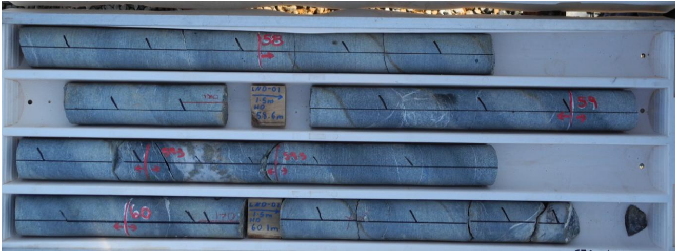
Figure 3 Core from Hole DVD037 showing 0.2m at 24.99 g/t from 59.3 metres.
