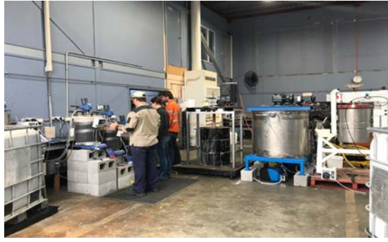
Figure 1: Pilot Plant – Solution Neutralisation Fe/Al removal tanks (left) including thickener and filter press (right)
